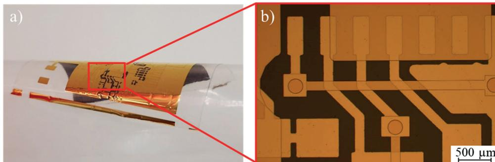
**Photo (a) and microscopic image (b) of an ultra-thin flexible Parylene-based printed circuit board with two metallization layers of gold.**
