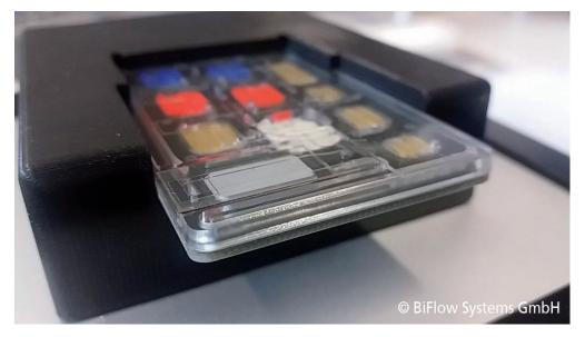
Microfluidic cartridge for the automated and miniaturized liquid handling with integrated micro pumps and heating elements. Photo © BiFlow Systems GmbH
