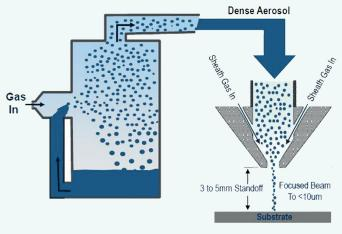
stream is deposited onto the substrate creating features as small as 10  $\mu$ m in size with a good and long-term stable adhesion. The maximum line width is around 200  $\mu$ m and depends mainly on the tip size and the gas flow parameters. At least the velocity of the printing process is up to 200 mm/s. Therefore also complex designs could be printed within a reliable time.
