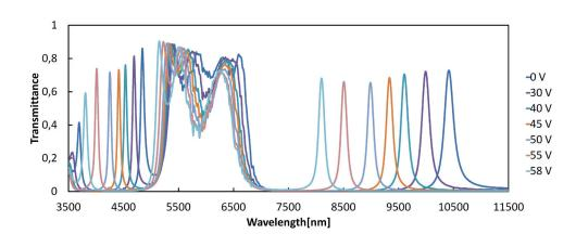
Fig. 1: measured transmittance spectra of a dual-band Fabry-Pérot interferometer for different control voltages. The wavelength ranges from 4 μm to 5 μm and from 8 μm to 10.5 μm can be used simultaneously.
