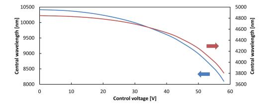
Fig. 2: Central wavelength as a function of control voltage on the example of a dual-band Fabry-Pérot interferometer for the wavelength ranges from 4 μm to 5 μm (red curve) and from 8 μm to 10.5 μm (blue curve).
