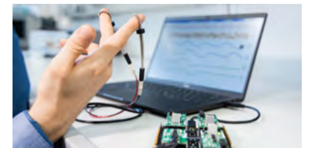
Finger exercise: Sensors measure the electrodermal activity (EDA) of the skin, which can play a role in stress monitoring, among other things.
