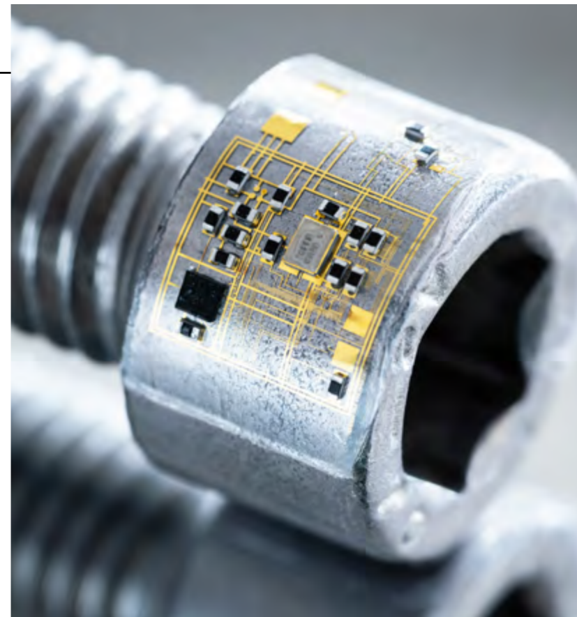
Flexible options: An ultra-flexible printed circuit board has been attached to the round head of a screw.
