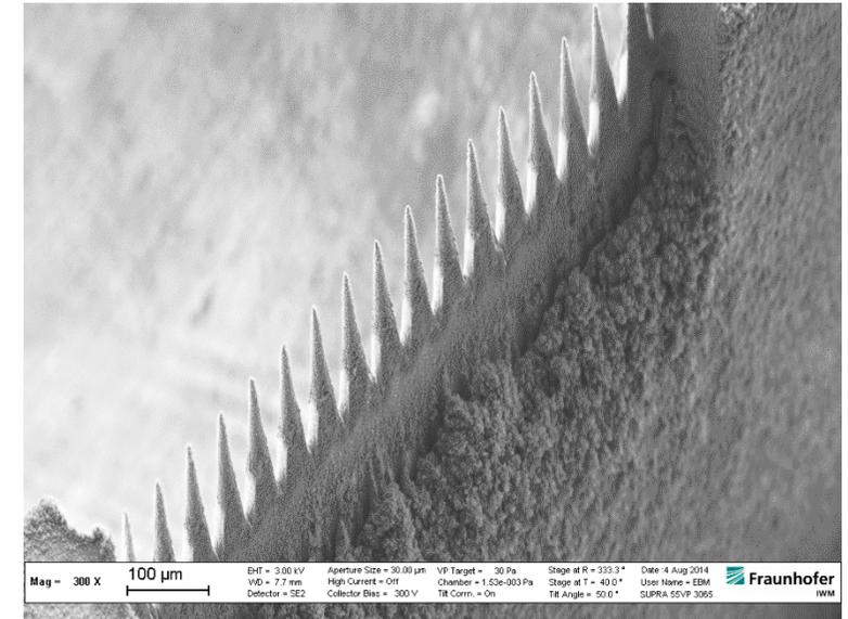
Automated preparation of a pillar array
