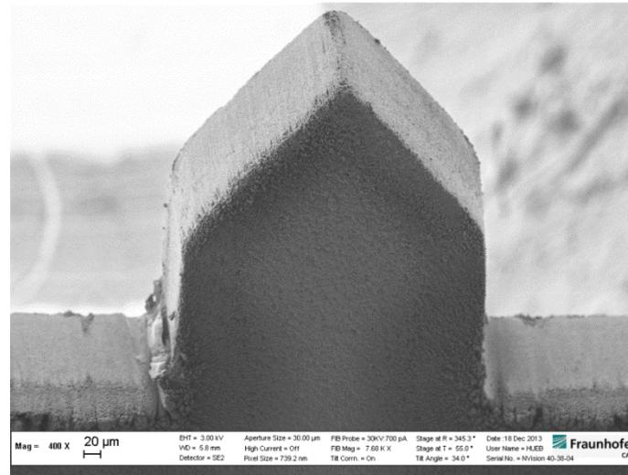
Tomographic basic structure laser-machined into silicon
