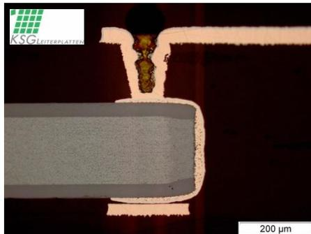
cross section of a buried capacity with connection
