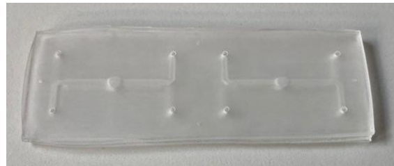
Two-channel chip with integrated membrane for barrier models
