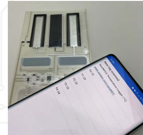
Printed Temperature Logger on PET
