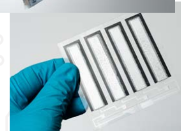
Printed Temperature Logger on PET
