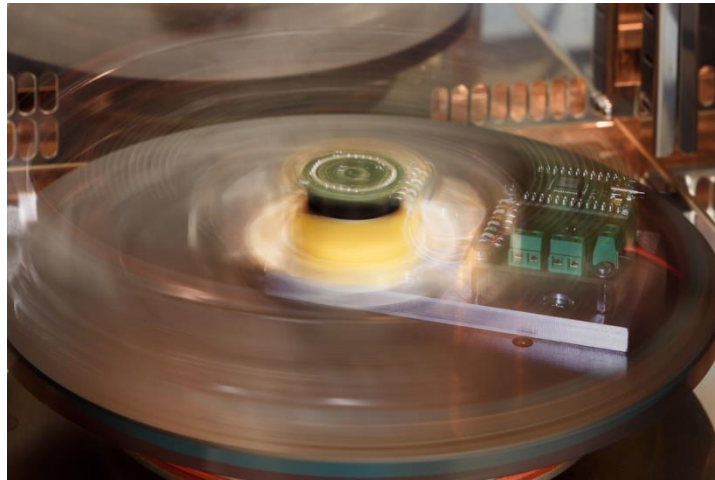
Rate table with horizontal and vertical axes in temperature chamber
