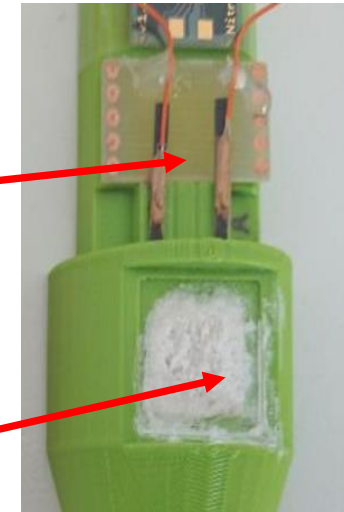
Soil tension sensor with conductive carbon wires on paper
