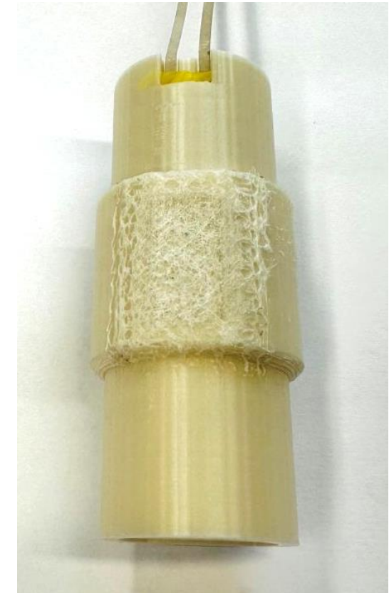
Soil tension sensor with conductive carbon wires on paper
