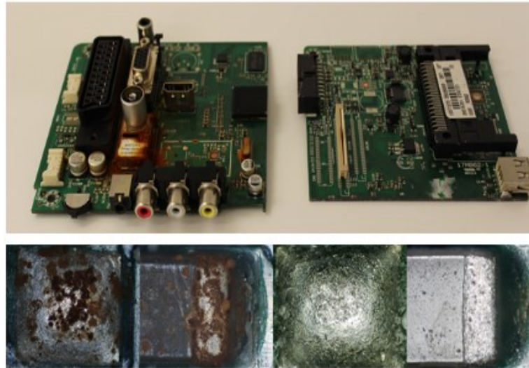
PCB with and without 5 µm Parylene C coating soaking for 1 week in 5 m% salt solution
