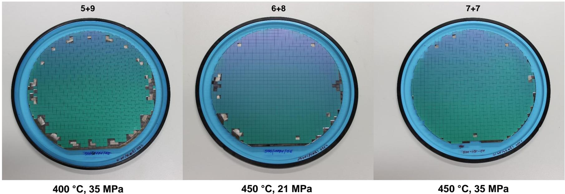
Nearly 100% dicing yield → missing chips on the edges should not have been bonded due to current collectors
