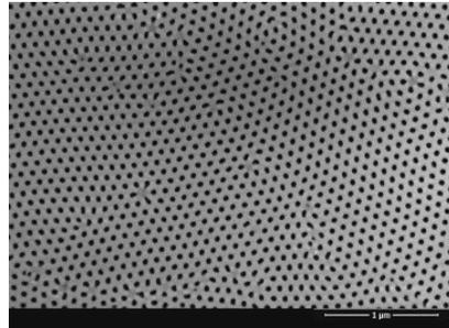
anodized ECD-Al (ECD @ENAS, Oxidation @ Smart Membranes)
