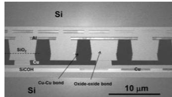
AI-TSVs for MEMS applications and hybride wafer bonding with Al
