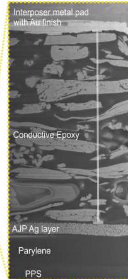
FIB cross-sections showing the relation of multilayer mesh and metal tap for interconnection towards PCB
