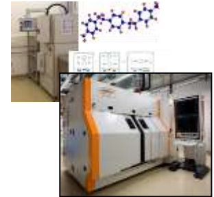
Thin film encapsulation/insulation by CVD to passivate 1 st Ag layer ( \sim 2\mu\text{m} ) and laser ablation to open vias
