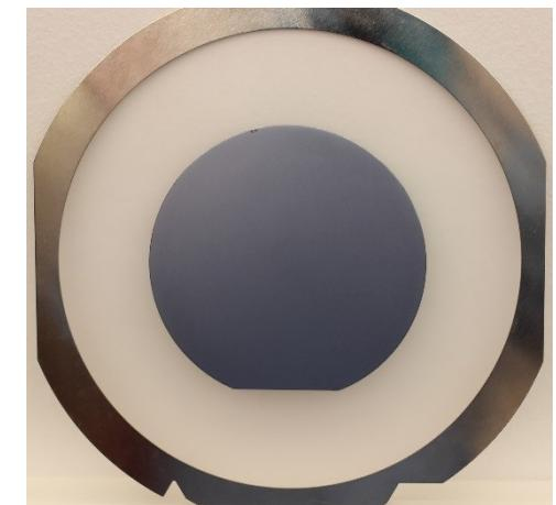
Fig.: wafer stack attached on dicing frame
