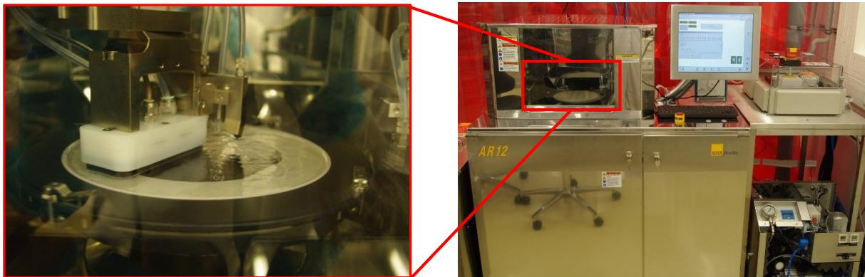
Fig.: edge release process in AR12 cleaning system
