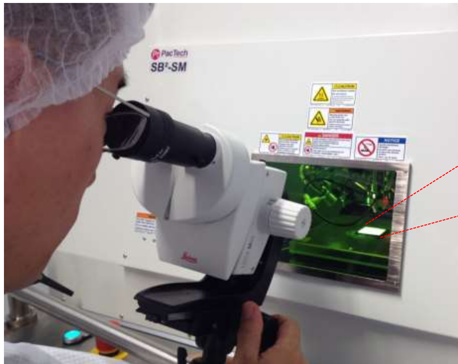
Solder Sphere Jetting (50 \mu\text{m} Spheres)
