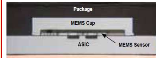
InvenSense ITG-3200 cross-section (Courtesy of System Plus Consulting)
