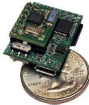
Fig. 2. EDA sensor module. The device has a modular design and is shown with an optional radio transceiver mounted on top.
