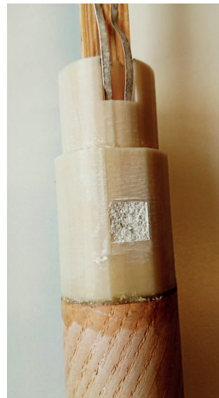
Soil moisture sensor made of biodegradable and inert material.
