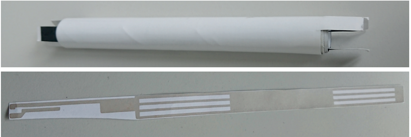
Printed components: printed battery (top) and printed antenna (bottom).
