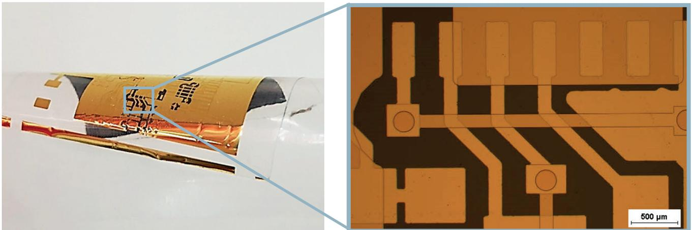
Photo and light microscopic image of the fabricated ultra-thin flexible Parylene PCB with two RDs.
