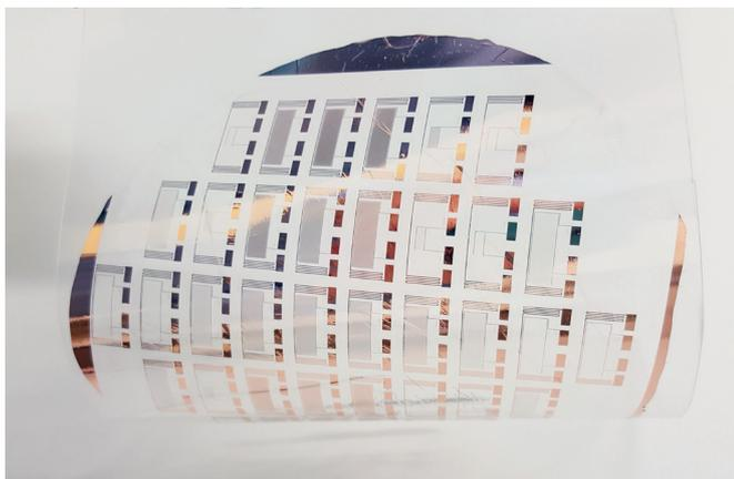
*Flexible Parylene substrate metallized by sputtered and wet-chemically etched copper.*
