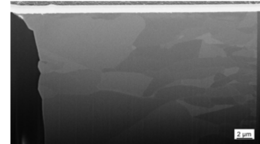
FIB preparation of 30 \mu\text{m} thick Al layer on highly doped Si
